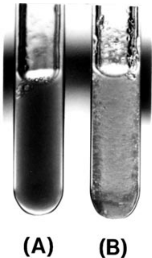
FIG. 2. Effects of the second heating in the presence of NaCl on the transparency of the soybean extract dialyzed against distilled water (A) and dialyzed and heated at 90°C under salt-free condition was heated again (B). Protein concentration, NaCl concentration, and pH were 75 mg/mL, 0.2 M, and 7.5, respectively.
